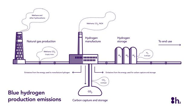
Figure 1. Greenhouse gas emission generated in the process of generating blue hydrogen.
